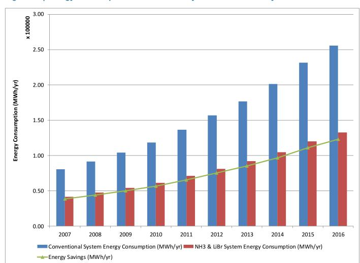
Figure 32 | Energy Consumption: Conventional System vs NH3/LiBr System
